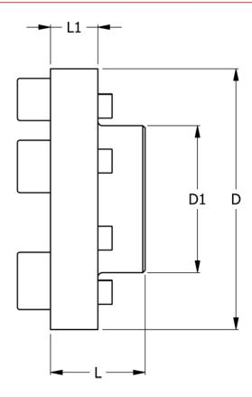
D = 660 D1 = 384 L = 260 L1 = 96 Max bore = 240 Torque (N m) = 49000
